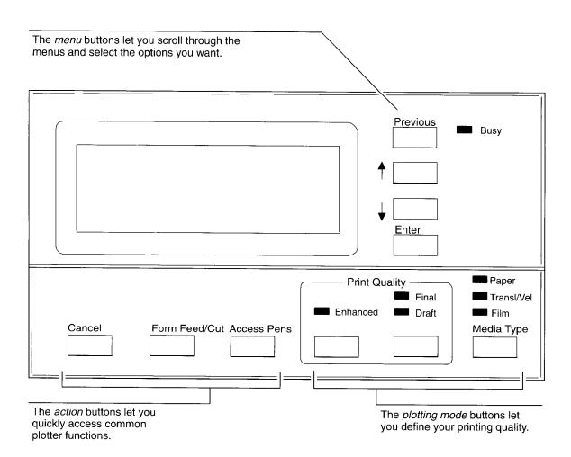
Virtually all interaction with the plotter involves using the front panel. The front-panel display shows several different types of information.
