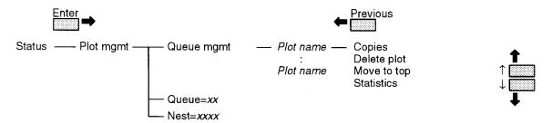
The plotter's queueing feature lets your plotter accumulate incoming plots in a list, or *queue*. After you place the plot file in the plotter's queue, you can change the order of plots in the queue, delete a plot from the queue, or change the number of copies the plotter makes. Nesting allows the plotter to place plots side-by-side to reduce the amount of wasted roll media (plots cannot be nested on sheet media).
